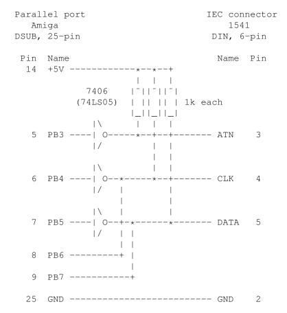
The 7406 (a 74LS05 will do as well) must be connected to +5V and GND of course. The trained technician will notice that this is the same
